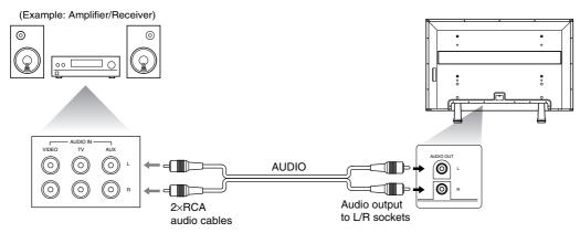
Connect the AUDIO OUT from the plasma display to the AUDIO IN on the amplifier/receiver.
